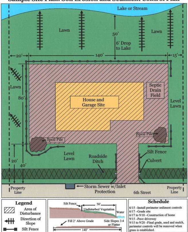
Sample Site Plan: Soil Erosion and Sediment Control Plan
